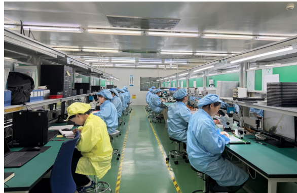
Seikoh Xunjie OFC mass produces MT fiber arrays in a clean room.
